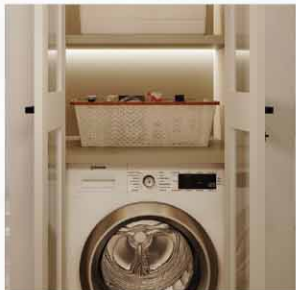
Washing Machine, Custom made wall and base MDF cabinets with mat lacquered paint finish.
